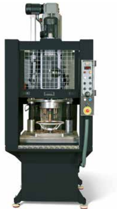
Drilling unit with a multiple head for steering wheels in the automotive sector, following the client's strict technical and safety standards.
