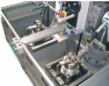
Detail of hydraulic self-centring clamping tools for automotive ball joints.
