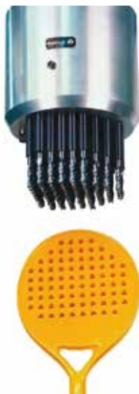
Simultaneous drilling application of 76 holes in a paddle.
